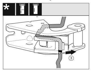
Remove the cable with the cable holder from the swap bearing block. Fig. 18 (3)
