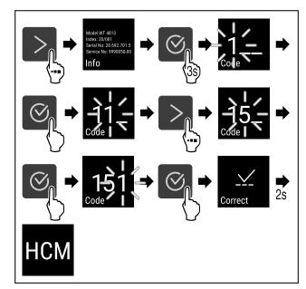
Fig. 6 Access with numerical code 151
