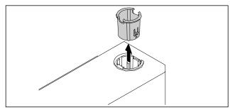
▶ Pull out the hinge bushing on the opposite side.
