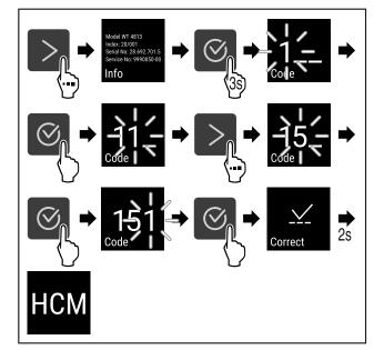
Fig. 6 Access with numerical code 151
