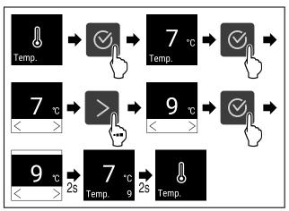
Fig. 68 Changing temperature from 7 °C to 9 °C
