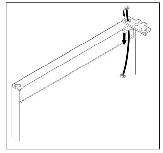
Fig. 43 ► Carefully push the cable through.
