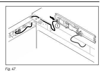
Connect the plug *Fig. 47 (1)* to the circuit board.
