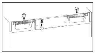
*Fig. 3 Example illustration* **(1)** LAN interface
