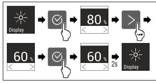
Fig. 101 Example illustration: Switch from 80 % to 60 %.
