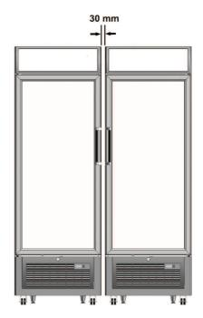
If several appliances are installed next to each other, leave a gap of 30 mm between them. If this gap is too narrow, condensation forms between the side walls.
