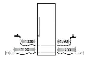
Fixed water connection (3/4") required for automatic ice-cube maker. Reinforced flexible hose (3m) for appliances with a 3/4" plumbed-in connection.
