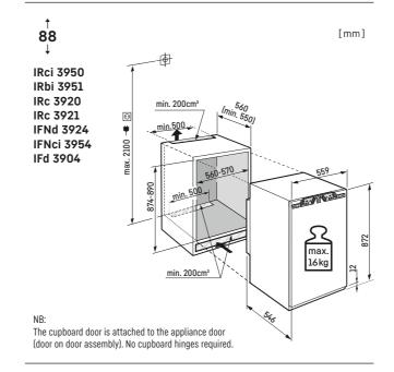
Please note that the recommended furniture door thickness limits are 16 mm–19 mm. Thicker door panels can be fitted within the relevant weight limits but specialist advice should be obtained. Please refer to the installation instructions for the individual model door weight limits.
