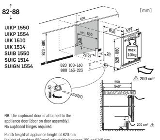
(height of worktop 850 mm) adjustable between 100 and 160 mm, or between 163 and 223 mm at appliance height of 880 mm (height of worktop 900 mm). Depth of plinth 22-77 mm.
