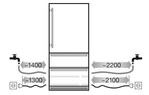
Fixed water connection (3/4") required for automatic ice-cube maker. Reinforced flexible hose (3m) for appliances with a 3/4" plumbed-in connection.
