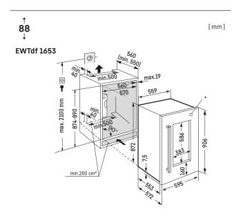
\* Shown with stainless steel frame installed. Door dimensions (w/h/d): 595/906/19mm.
