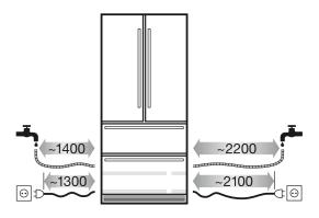
Fixed water connection (3/4") required for automatic ice-cube maker. Reinforced flexible hose (3 m) for appliances with a 3/4" plumbed-in connection.
