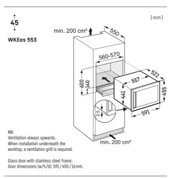
Please note that the recommended furniture door thickness limits are 16 mm-19 mm. Thicker door panels can be fitted within the relevant weight limits but specialist advice should be obtained. Please refer to the installation instructions for the individual model door weight limits.
