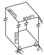
► Then prop up the door: Turn the adjustable foot on the bearing bracket (B) using the open-ended wrench SW10 until it comes into contact with the floor, then turn an additional 90°.
