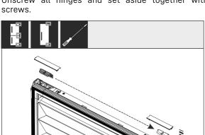
Fig. 14► Loosen and shift the bracket at the top and bottom of the door. The bracket must be shifted so you can screw on the hinges.
