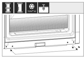
Shift the screws to fasten the hinge. Do not screw tightly after shifting – you need to hang the hinges later.
