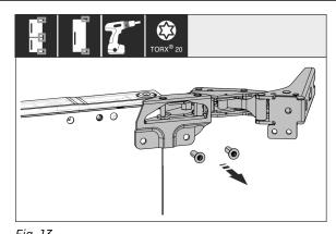
Unscrew all hinges and set aside together with the screws.
