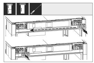
Fig. 16Swap the fixing bracket to the opposite side.
