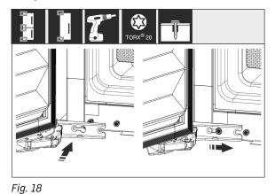
▶ Refitting the door: Hang the door with its hinges and tighten the screws.
