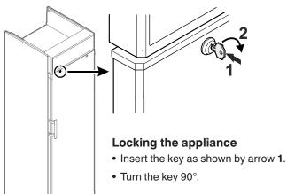
To unlock the appliance, the same procedure must be repeated in the same order.
