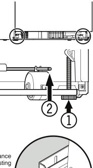
2. Adjust the height of the appliance at the rear by turning the adjusting bars ②.
