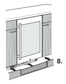
Fit the plinth panel. In doing so, the foam moulding is pushed backwards into its final position.
