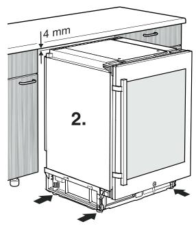
Adjust the height of the appliance to 4 mm less than the recess height by turning the adjustable feet clockwise.
