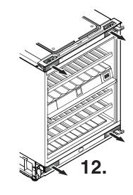
8. Compress the covers in the places shown and release. Turn the covers through 180° and click into place on the opposite side.
