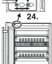
24. Undo screws and slide hinge bracket to the right or left.
