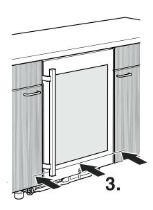
3. Slide in the appliance until the front surface of the appliance door is flush with the unit fronts.
