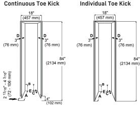
Cabinet depth frameless installation style = 25" (635 mm) Cabinet depth inset installation style = 25" (635 mm) + panel thickness
