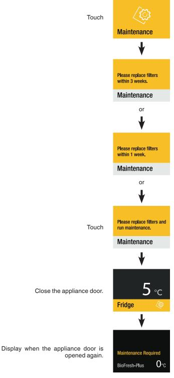
Obtain water filter and air filter from your dealer and complete the maintenance procedure.
