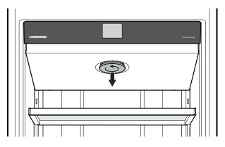
Turn the cover anticlockwise and remove it.
