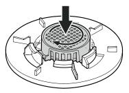
If the water flow is no longer even, the aerator must be replaced (see contact details on the back of this manual).
