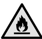
**WARNING:** Danger of fire / flammable materials. This symbol is located on the compressor and indicates the danger of flammable materials. Do not remove the sticker.
