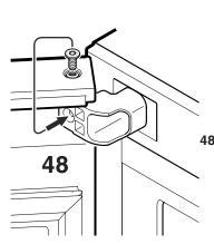
**48.** Undo screw in hinge pin and screw into bore hole in hinge bracket.
