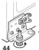
**44.** Insert pin fully into hinge bracket and tighten adjustable foot by hand.
