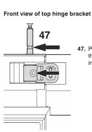
**47.** Push in hinge pin until groove in the pin lines up with bore hole in the hinge bracket.
