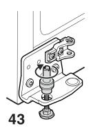
**43.** Fit adjustable foot from underneath and attach hinge pin to it.
