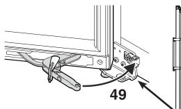
**49.** Move soft stop mechanism hinge to the fastener.
