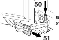
50. Insert pin.51. Remove red safety bracket.
