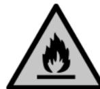
The symbol is located on the compressor and indicates the danger of inflammable materials. Do not remove the label.
