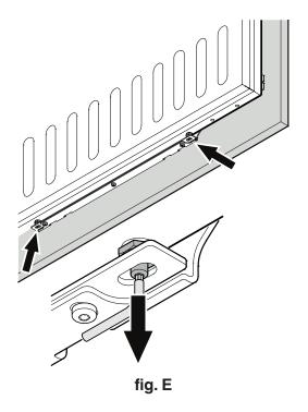
Undo the three screws on the top of the attachment bracket, adjust the door panel as displayed in fig. G and then retighten the screws. The same procedure can be carried out for the bottom attachment bracket.
