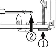
2. Adjust the height of the appliance at the rear by turning the adjusting bars (2).
