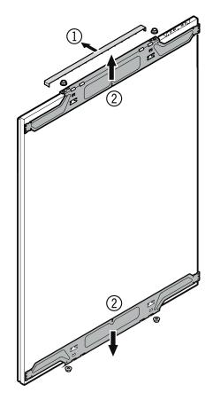
Unscrew the attachment brackets (3) from the freezer drawers. These attachment brackets will be mounted onto the freezer panels.
