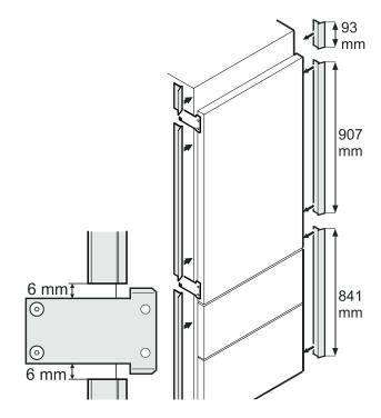
Apply the cover strips 6 mm from the securing plates.
