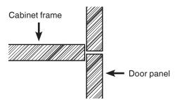
Min. panel thickness = 16 mm Max. panel thickness = 38 mm
