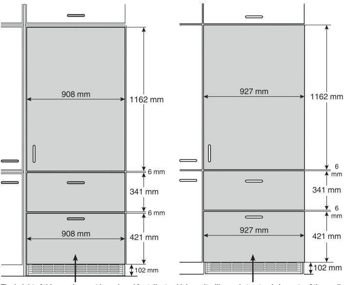
The height of this panel cannot be reduced for taller toe kicks as it will reveal structural elements of the appliance. Instead, install appliance on a platform and adjust the opening height to accommodate.
