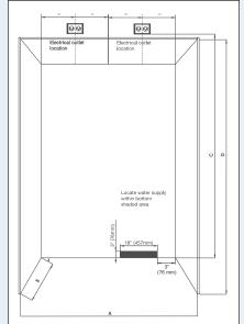
\*The given cabinet opening height dimension includes space for top air vent. If you choose to place the vent above the cabinet or in a soffrt, you will need to adjust the height dimensions accordingly. Please refer to Ventilation
