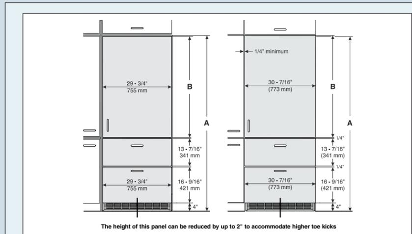
Minimum panel thickness is 5/8" (16 mm).
