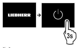
Fig. 3 ► Switch on the appliance using the display.
