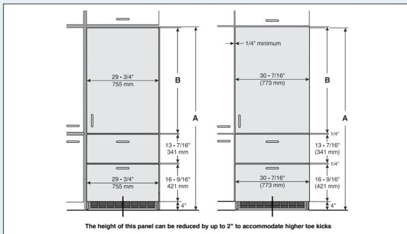
Minimum panel thickness is 5/8" (16 mm).
