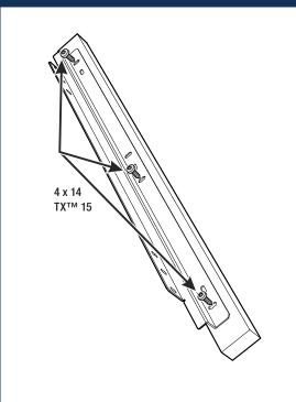
Mount the panel onto the angle bracket using three 4 x 14 screws.
