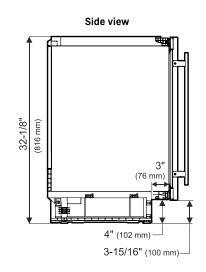
23 - 5/8" (600 mm) min. 24" (610 mm) max. Lim (610 mm) max. Counter depth dimension without cabinet door 22 - 3/4" (578 mm)
