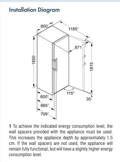
Important information: For Side-by-Side installation the freezer or the appliance with freezer compartment must be installed on the left as viewed from the front to prevent possible formation of condensation.
