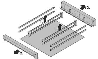
► To disassemble the cabinet:Lift the inner retaining rods upwards, pull the brackets out. This releases the front and rear retaining rods as well as the glass panel.
