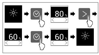
Fig. 50 Example illustration: Switch from 80 % to 60 %.
