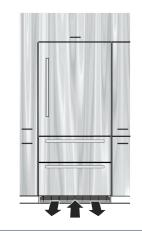
The appliance do not require ventilation considerations in the cabinetry. The required airflow is directed through the toe kick base. It is important to use the provided cover grille for the ventilation opening. This opening must not be covered.
