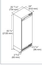
IMPORTANT! Stated minimum height dimensions include when the leveled feet are fully inserted.
