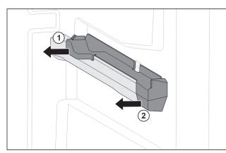
Fig. 73 Attachment on the right moulded rib
