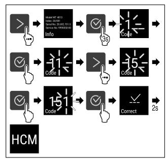
Fig. 6 Access with numerical code **151**
