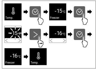
Fig. 65 Changing temperature from -15 °C to -16 °C
