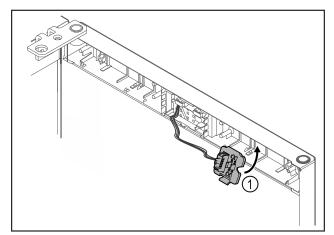
▶ Snap in the plug holder Fig. 21 (1) on the opposite side.
