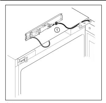
▶ Disconnect the plug *Fig. 16 (1)* from the circuit board.
