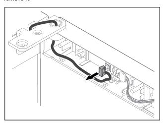
Fig. 19 ► Remove the plug from the plug holder.
