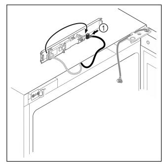
Fig. 17 ► Connect the plug *Fig. 17 (1)* to the circuit board.
