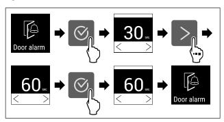
Fig. 111 Example illustration: Switch door alarm from 30 seconds to 60 seconds.
