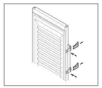
Fig. 28 Insulated door Remove the panels. Unscrew the handle.
