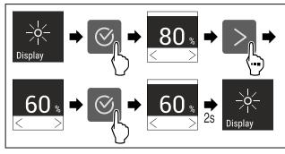
Fig. 83 Example illustration: Switch from 80 % to 60 %.
