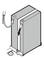
Plug the connector onto the positive pole on the battery.
