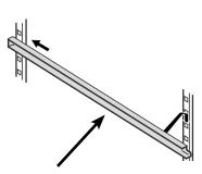
Suspend the rails at the desired height, by inserting into the rear clip-in strip first and then clipping in at the front.
