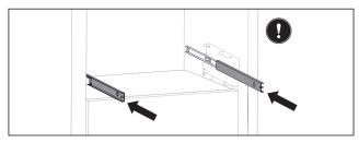
If the rails are not yet fully inserted after removing the drawer:
