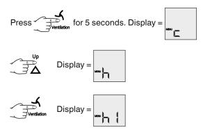
Use buttons Up and Down to select the desired setting.
