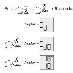
The refrigeration unit switches on. The temperature display flashes.
