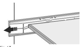
Fig. 6 \*▶ Pull off the transport lock on the appliance door.
