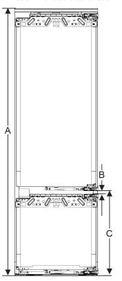
Fig. 64 Clearances for a 2-door cabinet door
