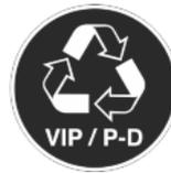
A sticker to this effect may be applied to the rear of the appliance. It refers to the foam-padded panels in the door and/or the housing. This is only relevant for recycling. Do not remove the sticker.
