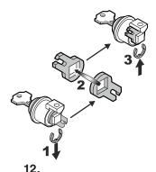
Remove door latch, turn over and re-assemble.
