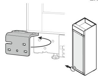
21. Turn the hinge bracket to the right. This tensions the spring in the closing mechanism.
