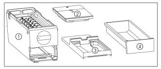
Fig. 76 Components of the EasyTwist-Ice
