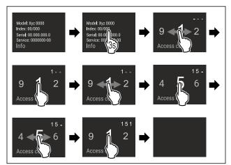
Fig. 3 Example illustration, access with numerical code 151
