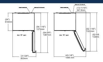
Allow door swing clearance at locations next to a wall. If the appliance is installed with the hinges next to a wall (4), the distance between the appliance and the wall must be at least  $\frac{1}{2}$ " (13 mm.)
