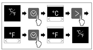
*Fig. 19 Example illustration: Switch from degrees Celsius to degrees Fahrenheit.*
