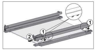
*Fig. 104 Glass shelf with rails and retaining parts* Install rail **with** damping mechanism:
