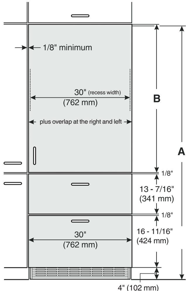
Product also allows installation with Toe kick height of 2" (50mm) to 6 11/16" (170mm).
