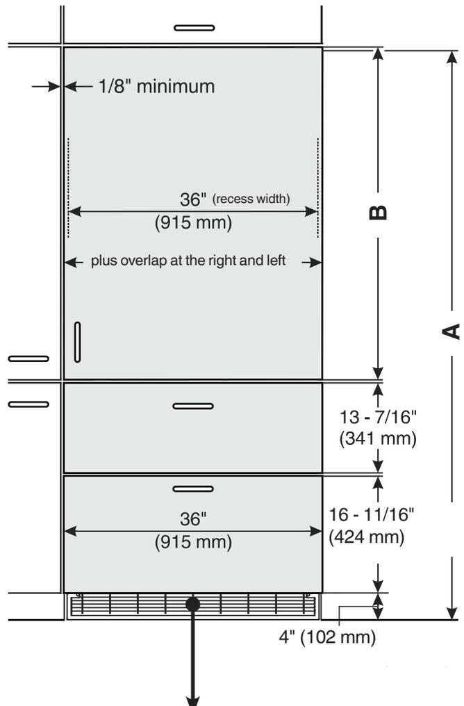
The height of this panel cannot be reduced for higher toe kicks as it will reveal structural elements of the appliance. Instead, install appliance on a platform and adjust the opening height to accommodate.
