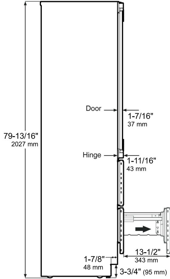
Height can be increased by 1-1/2" (40 mm) by turning the levelling feet at the front and the height adjustable roller units at the appliance rear.
