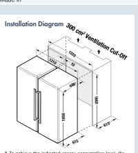
1 To achieve the indicated energy consumption level, the wall spacers provided with the appliance must be used. This increases the appliance depth by approximately 1.5 cm. If the wall spacers are not used, the appliance will remain fully functional, but will have a slightly higher energy consumption level.
