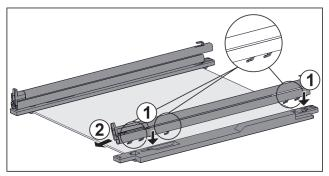
Fig. 69 Glass shelf with rails and retaining parts Install rail with damping mechanism:
