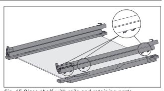
Fig. 65 Glass shelf with rails and retaining parts The rail hooks are released from the retaining part.
