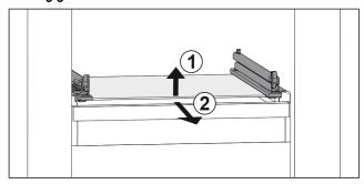
Fig. 51 Example illustration of glass shelf
