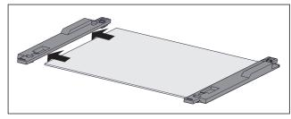
Fig. 66 Glass shelf with retaining part
