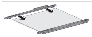
Fig. 67 Glass shelf with retaining part
