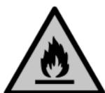
This symbol is found on the compressor and indicates the danger of flammable materials. Do not remove the sticker.
