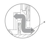
A gap of 1 3/8" (35 mm) must be maintained to ensure sufficient ventilation.
