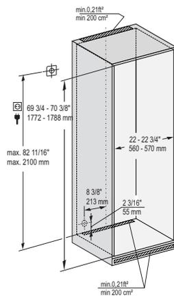
This is a fully integrated wine appliance designed to be completely enclosed in a dedicated kitchen cabinet. This dedicated cabinet box must be constructed in accordance with the specified dimensions and must allow for sufficient air circulation to ensure proper operation. For more details about ventilation requirements, please refer to the Design Guide.
