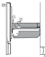
The bottommost freezer drawer must be removed to clean the glass plate in the freezer compartment.
