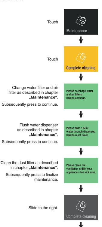
Obtain water filter and air filter from your dealer and complete the maintenance procedure.
