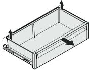
Pull the freezer drawer upwards by its right and left bottom corners (1).
