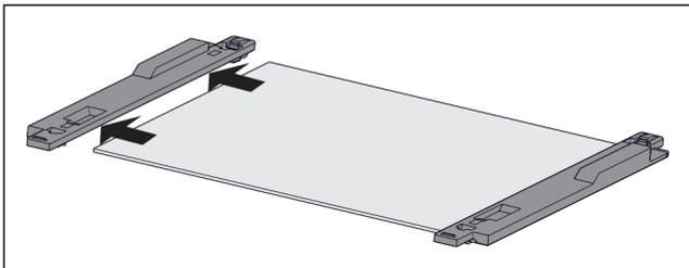
Fig. 45 Glass shelf with retaining part
