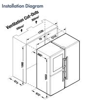
1 To achieve the indicated energy consumption level, the wall spacers provided with the appliance must be used. This increases the appliance depth by approximately 1.5 cm. If the wall spacers are not used, the appliance will remain fully functional, but will have a slightly higher energy consumption level.
