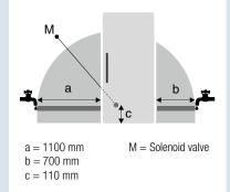
Plumbing must be installed adjacent to the side of the appliance which contains the IceMaker.
