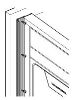
Fasten the appliance in the recess through the appliance cover strips using eight screws 4 x 14 for each side. We recommend that you mark and pre-drill the hole positions in the strip.
