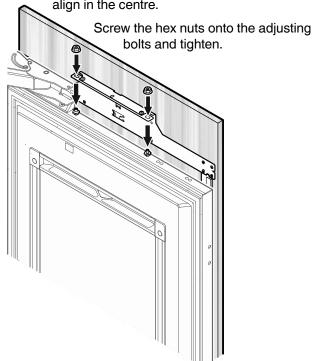
Close the door and check the position of the panel.
