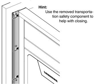
Push the mounting strip upwards. The bottom edge of the mounting strip must be aligned with the top edge of the adjacent cabinet door.
