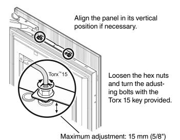
Align the panel horizontally with the long holes in the attachment bracket.
