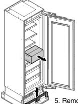
4. Remove the box with mounting parts.
