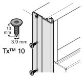
Apply the appliance cover strips to the left and right front edge of the appliance housing, align in height with the top profile and screw into place. The strip is transparent so the designed mounting holes on the appliance housing are visible. We recommend that you mark and predrill the hole positions in the strip.
