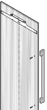
Only use countersunk screws for handle mounting.
