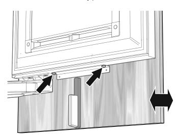
Fasten the panel through the bottom attachment bracket with two screws 4 x 14.
