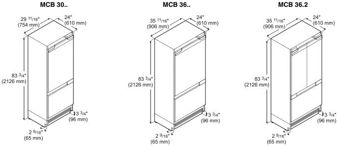
Stated minimum height dimensions include when the levelled feet are fully inserted. Width will increase by 1/4" (6.5 mm) when mounting strips are installed.
