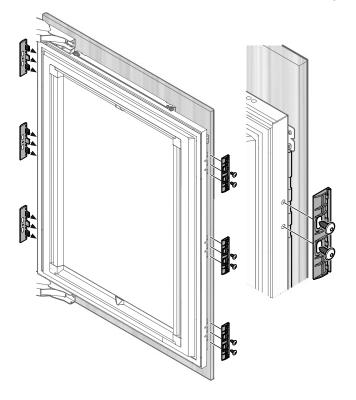
Hook the door cover strips at the front of the supports and snap in at the back.
