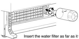
Insert the water filter as far as it will go with the front knobs in a horizontal position and turn clockwise until it snaps in.
