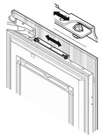
Align the panel horizontally with the long holes in the attachment bracket.
