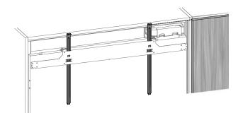
Open the door. Unscrew the attachment bracket with the mounting strips.
