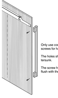
Only use countersunk screws for handle mounting.
