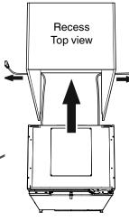
IMPORTANT After sliding the appliance into the recess, plug in the appliance and check its function. Then unplug it again.
