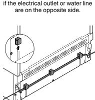
Install the cable holders on the rear of the appliance. Insert power cord/ water line in cable holders.
