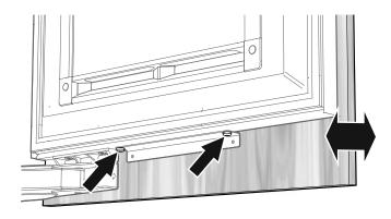
Insert the panel supports into the support strips between panel and appliance door and screw into place with two screws M6 x 12 each.
