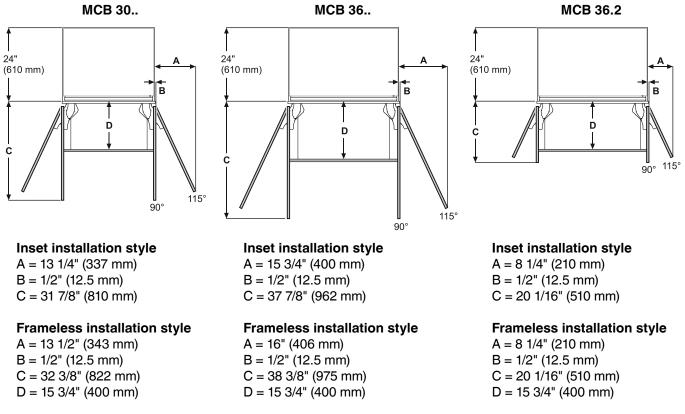
Dimension A and B: Add panel thickness and handle to calculate distance to wall.
