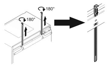
Remove the mounting strips, turn them through  $180^\circ$  and insert them as far as possible into the attachment bracket.
