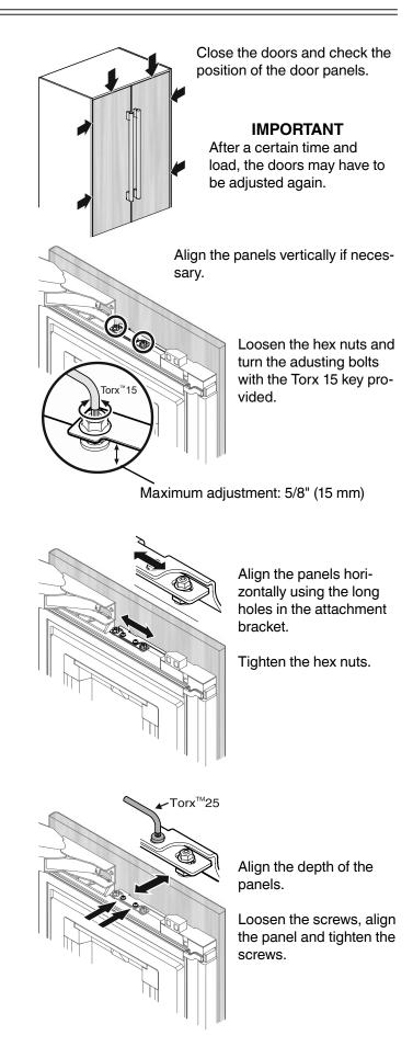
Align the panel in its depth at the bottom.
