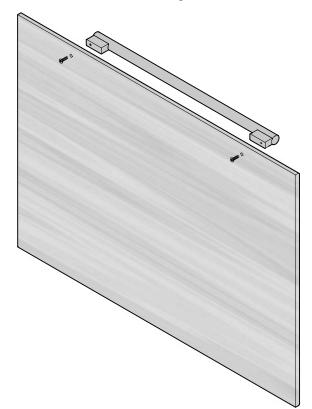
Only use countersunk screws for handle mounting.
