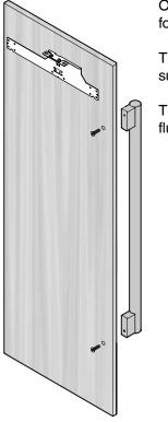
Only use countersunk screws for handle mounting.
