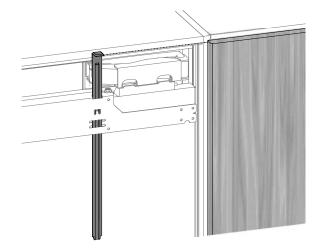
Open the door. Unscrew the attachment bracket with the mounting strip.
