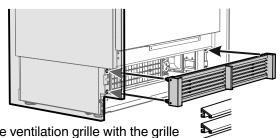
Mount the ventilation grille with the grille segments tilted down.
