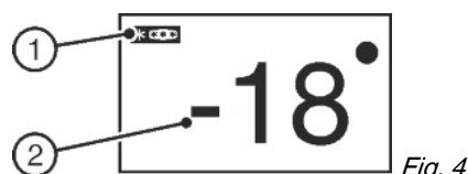
Fig. 4 (1) Freezer compartment symbol (2) Freezer compartment temperature display
